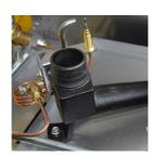
90° venturi that prevents the nozzle from clogging and accumulating dirt.
