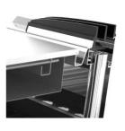
Plate not welded to the machine bed with optimisation of structural points under thermal stress
