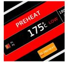
The PREHEAT function allows you to preheat the griddle in order to reactively cook dishes. by setting a set temperature, the equipment will set a higher temperature delta to compensate for the lowering due to the positioning of the dish
