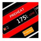
The PREHEAT function allows you to preheat the griddle in order to reactively cook dishes. by setting a set temperature, the equipment will set a higher temperature delta to compensate for the lowering due to the positioning of the dish
